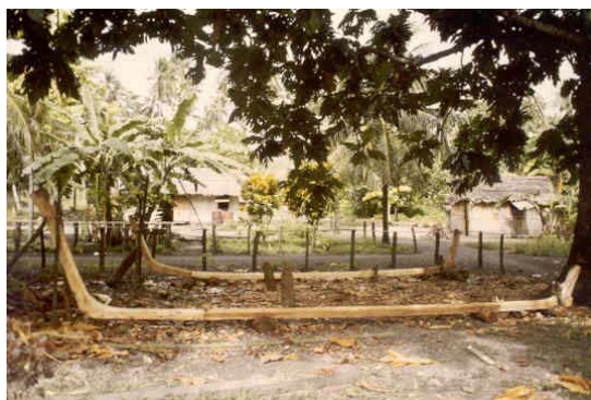
Keel beam with prow and stern post of a boat under construction.
